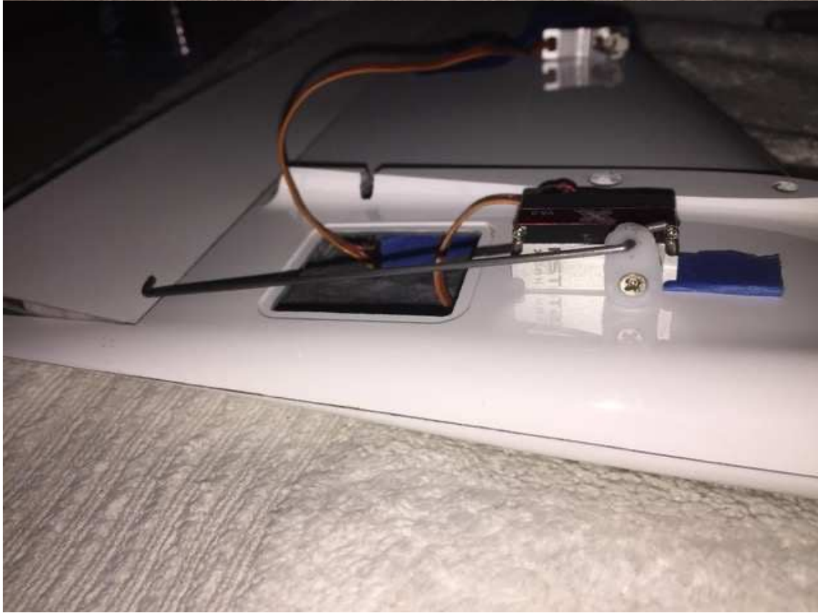
Rudder servo: Mount the rudder servo on its frame and cut the wire to the correct length as shown in the picture. With the servo checked as in the neutral
